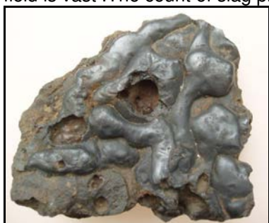
Fig 18 .Typical sample of iron slag produced in the Iron Age and Roman times .
